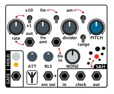
Voices are triggered using a pushbutton keyboard, particularly buttons 3 and 8, creating a 5V gate that triggers the Attack/Release envelope, opening the VCA in the voice. External CV sources can be used to trigger the voice, driving the envelope. The output of the envelope can be used to trigger the next voice or to modulate the voltage on the filter or the effector.
