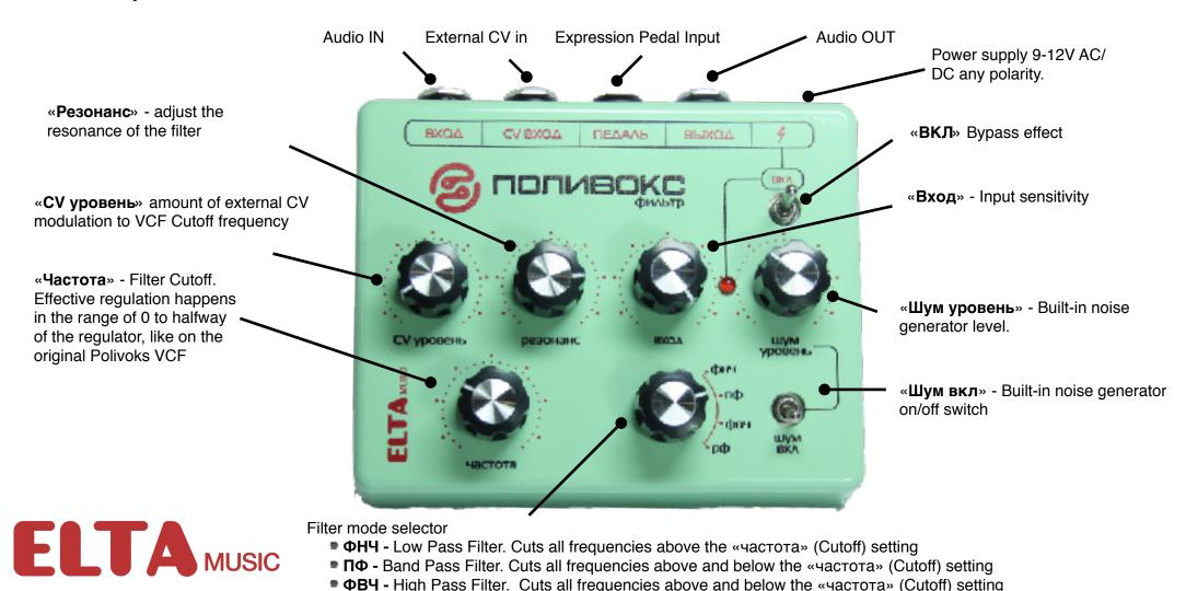
■ РФ - Notch Filter. Cuts the narrow frequency band near the «частота» (Cutoff) setting
